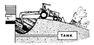
Level the backhoe on slopes with the stabilizers to dig plumb trenches, or use the backhoe or loader to cut a level slot for the uphill wheel and stabilizer. Pile the spoil from the slot on the low side.
